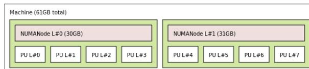
Notice that hwloc only sees half the PUs when SMT is disabled. PU L#6, for example, seems to change location from NUMA node #0 to #1. In reality, no PUs "moved" – they were simply re-numbered when hwloc only saw half as many (see also Logical index in [Indexes and Sets](#)). Hence, PU L#6 in the SMT-disabled picture probably corresponds to PU L#12 in the SMT-enabled picture.
